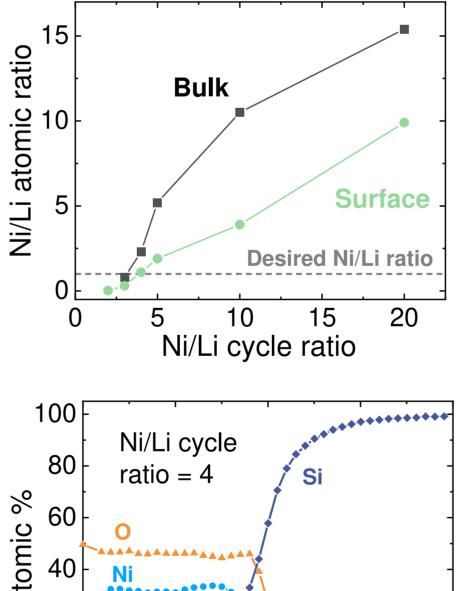
Depth profiles show **low levels of C and Si** contamination in the bulk.
